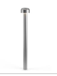
100-240V power supply included. Ready for installation on solid surface. Each luminaire is equipped with 200 mm cable for connection inside the luminaire body. Reccomended connection wit a 2 way terminal block 4 poles IP68 H2O Stop, to be ordered separately.
